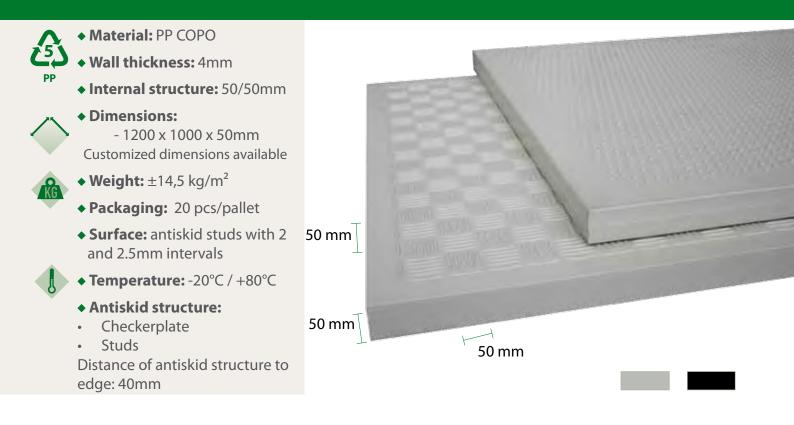
Paneltim<sup>®</sup>'s panel range includes two varieties of antiskid panels with a reinforced 50x50mm internal cell structure: a checkerplate and stud antiskid structure. Both types of panel are light, rigid and closed on all sides, which makes them easy to clean.
