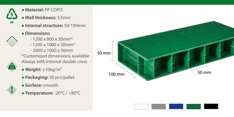
The 50mm lightweight panel with 50/100mm internal cell structure is highly suitable for dividers, stable doors, non-supporting walls, personnel doors,... In short any application which requires a light, strong and hygienic solution. The panel has a thick wall but is nevertheless light and rigid which makes it possible to realise large dimensions.
